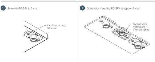
3 Options for mounting PC-SF1 to support frame and male clip and panel types
